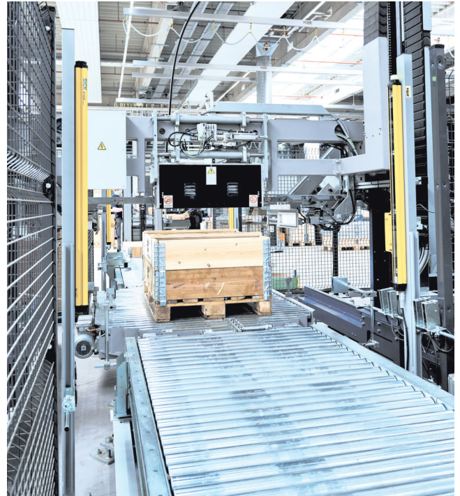
Fully automatic machine in end-of-line packaging
